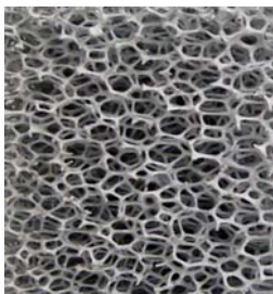
Fig. 1: 3D network structure of an open cell metal foam.
