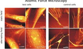
For all AFM images cantilevers with resonant frequency f=17 kHz and spring constant k=0.1N/m have been used in contact mode. Single actin filaments are visible. Comparison of cell height and thickness of the filaments of test and control cells show no significant difference. Signals between two cells are artifacts which occured during the drying process in methanol.
