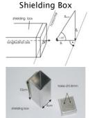
The mumetal box ( $\mu_r$ = 25000  $\Leftrightarrow$  shielding factor:  $A_{par}$ =500,  $A_{ort}$ =250) decreases the intern field to a maximum value of 180 nT (earth magnetic field 50 μT, angle of hade 66°).
