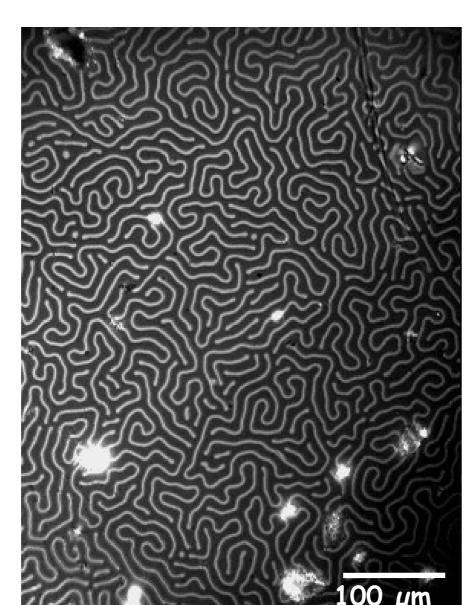
Faraday microscopy of a garnet film under the influence of different external magnetic fields
