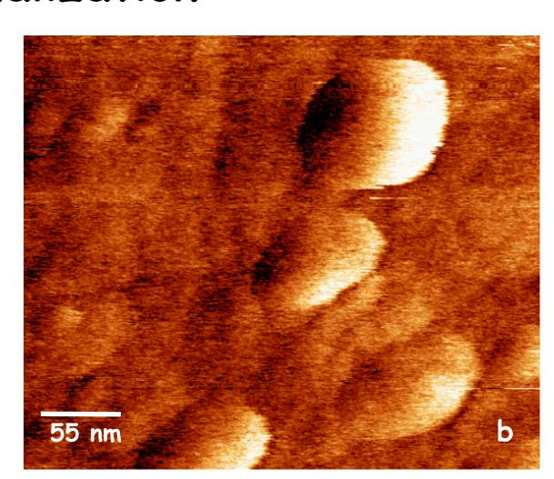
Magnetic force and atomic force microscopy are used to visualize single magnetic beads. The MFM technique gives information about the magnetic properties (stray field) of the beads or magnetic surface structures (not shown).
